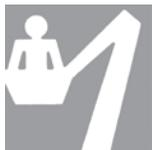
The work platform must have 1.1 metre high guardrails, comprising handrail, knee-rail and foot-rail on all sides, and a non-slip floor. The access door to the basket must close securely. The guardrails must also ensure that tools and similar items cannot fall from the work platform. Fall protection equipment must always be used when operating personnel lifts.
